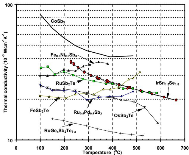
Figure 8: Thermal conductivity as a function of temperature for several ternary skutterudite compounds. Results are compared to those obtained for lightly doped CoSb<sub>3</sub>.
