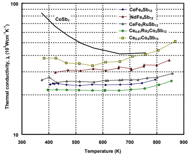
Figure 15: Thermal conductivity as a function of temperature for various Fe-, Ru-, and Co-based filled skutterudites. Results are compared to p-type CoSb<sub>3</sub> data.
