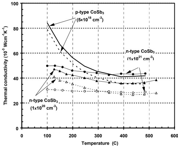
Figure 5: Lattice (dotted lines) and total (plain lines) thermal conductivity as a function of temperature for CoSb<sub>3</sub> samples with various doping levels.
