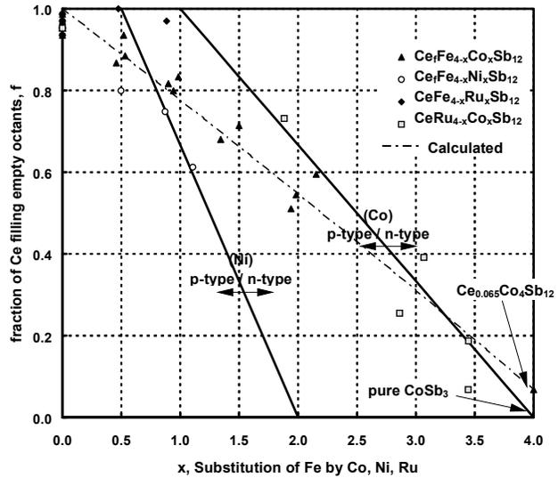
Figure 13: Ce filling fraction (f) for  $\text{Ce}_f\text{Fe}_{4-x}\text{M}_x\text{Sb}_{12}$  samples as a function of Fe substitution by M (x) with M = Co, Ni and Ru. No decrease in Ce filling is observed for  $\text{Ce}_f\text{Fe}_{4-x}\text{Ru}_x\text{Sb}_{12}$  samples.
