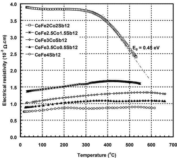
Figure 9: High temperature variations of the electrical resistivity of p-type  $\text{CeFe}_{4-x}\text{Co}_x\text{Sb}_{12}$  filled skutterudites.
