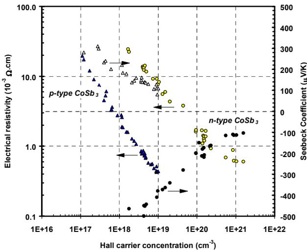
Figure 3: Room temperature electrical resistivity and Seebeck values as a function of carrier concentration for CoSb<sub>3</sub>.
