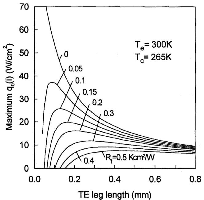
Figure 1: Maximum (by current density) cold side heat flux density versus TE leg length for different  $R_t$  values.
