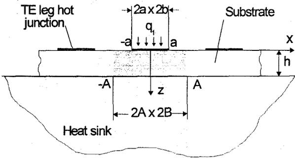
Figure 3: Scheme of TEC hot side substrate.
