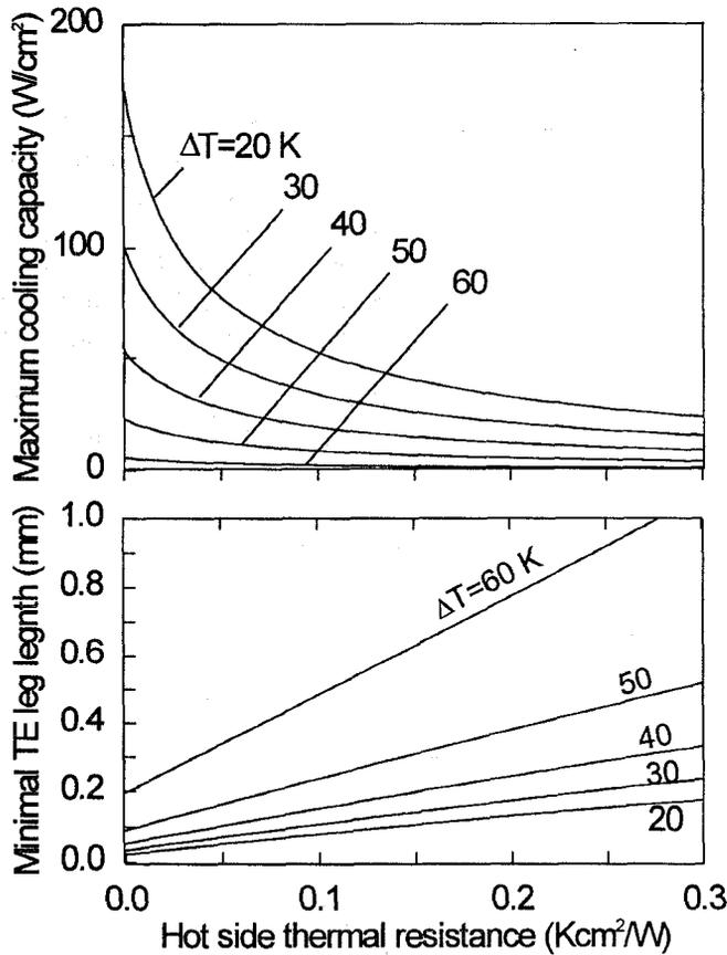
Figure 2: Minimal TE leg length and maximum cold side heat flux density versus hot side thermal resistance.
