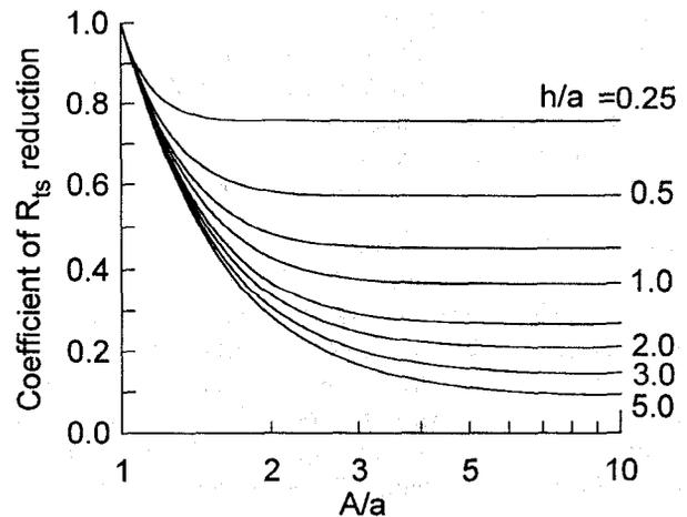
Figure 4: Reduction of substrate thermal resistance with TE legs spacing.
